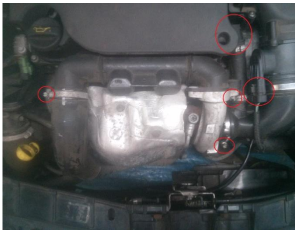
Remove engine cover and pipes.
