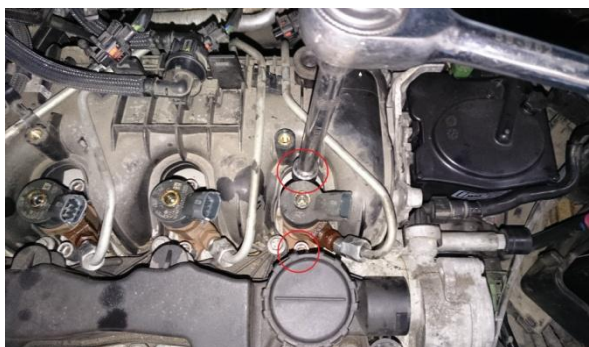
Remove 2xbolts, slide injector up.
