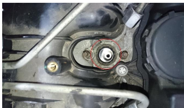
Shiny injector seat after cleaning
