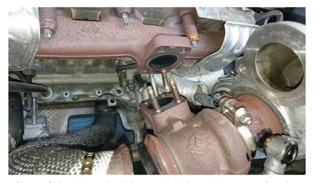
Before you refit the turbo, you will need the correct oil pipe (part number 9806878180 for PSA). We would also recommend fitting new banjo bolts at either end. Don't remove the strainer from the lower bolt, it's a filter and an oil restrictor, removing it will cause future problems. Attach the oil drain pipe before refitting the turbo, new drain pipe is 9686659280 038131 (for PSA). Gaskets 038036 and 038037 are required.
