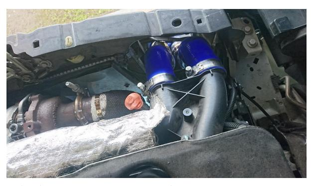
Here's the final job with the intercooler and pipe work fitted.
