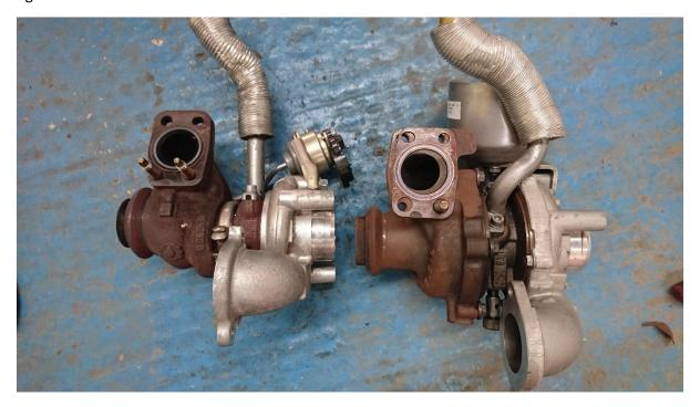
The position of the oil drain and the oil feed is the same, so it's quite an easy conversion. The exhaust fitment is also the same. The DPF can remain if you are using the car for road use. With a DPF fitted you will likely get less power than the quoted figures because it can cause a restriction.
