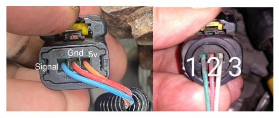
The important thing is to match the required position for the GTD12 turbo. \*Usually 1 and 3 should be swapped\* However, please check which pin is 5v using a multi meter.
