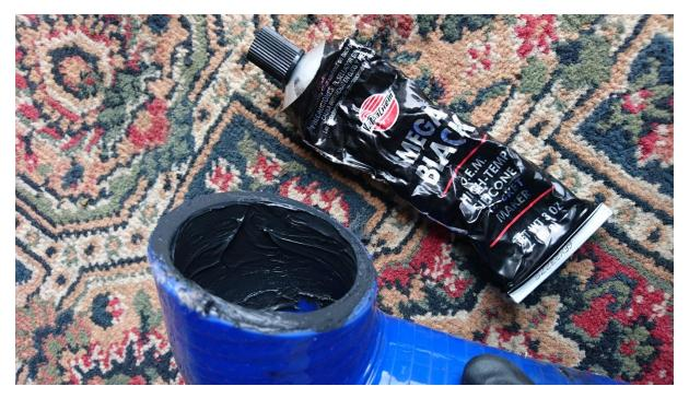
Use a jubilee clamp tightened over the opposite side of the flange on the turbo so that the pipe can never pop off. Let the silicone dry before testing the vehicle, you now have a very permanent seal on this hose that will not affect reliability.
