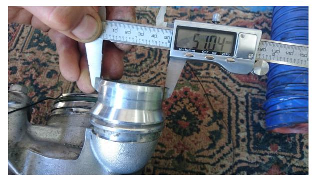
Although the end of the turbo outlet is 51mm, there is no way to secure a pipe on to this without finding the original BMW pipe with a tight radius and a locking clip. Flexible corrugated hose was tested, and this did not last long as the jubilee clamps wore through the hose, although the hose did not pop off.
