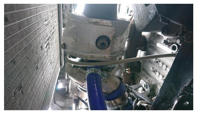
Join the silicone with a piece of 16mm tubing and then run it to a 16mm 90 bend. I chose to make this slightly short to keep the bend uphill rather than with a dip at the bottom which would fill with oil.
