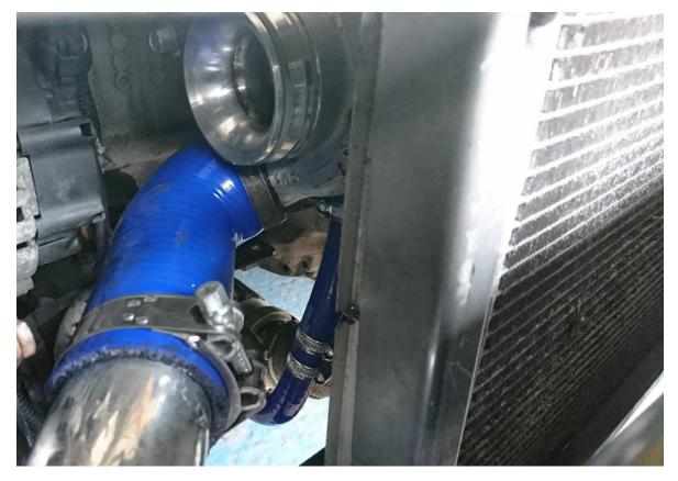
The turbo inlet fits a 76mm 90 hose which can be reduced to a 57mm hose. Run the pipe along the front of the engine bay over to a free flow air filter. There is no need to run a MAF on this build as we can calculate air mass through the ECU using the boost pressure reading, air temperature and the volumetric efficiency of the engine. The standard MAF will be maxed out at anything past 145 BHP so it doesn't serve much of a purpose on a build like this.
