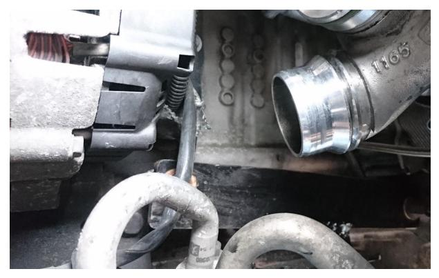
After making up a jig I could make a manifold adaptor and get the turbo in place. Here's one I manufactured myself using a MiG welder and very thick butt weld stainless fittings. Due to distortion after welding I needed to take this to a friend's machine shop to get the flanges perfectly flat so that they would make a nice seal. Use a new Peugeot gasket on one side and the BMW gasket on the other side to create a good seal.
