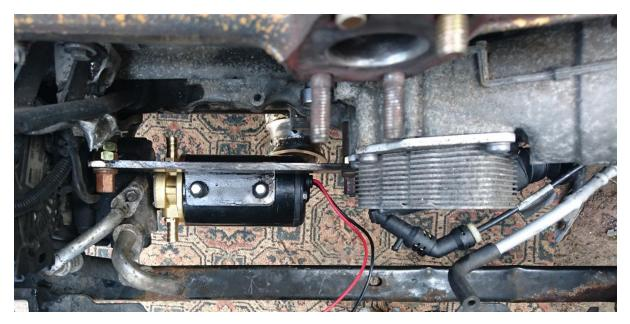
After realising that a new sump pan would cost only £30 if my next plan didn't work I took the sump straight off. I saved the oil I drained out and poured it in to the sump. The oil level with 4.5 litres came right to the top of the sump. As the turbo drain can't have any restrictions this at first worried me, but I quickly realised that with the engine running most of the oil would be pumped around the engine.
