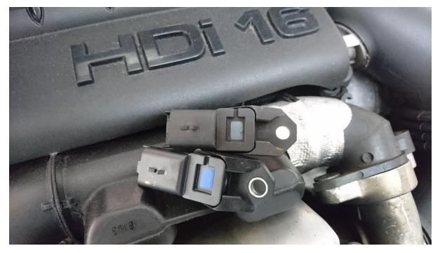
The plug is almost the same, but you'll need to scrape the side off to remove the slot which prevents it going to the sensor. For both the MAP sensor and the injectors it's important that you don't use the vehicle without having them calibrated in to the ECU through a remap.
