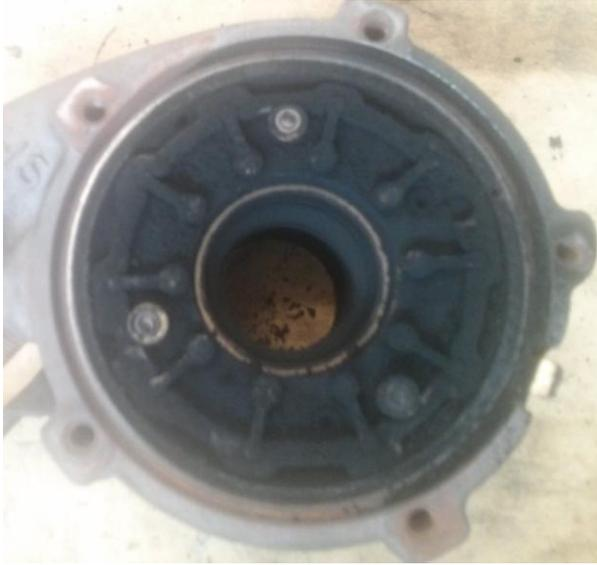
6. Lift the rollers out with a screw driver and then the VNT ring will lift off. Once off, you can also remove the roller pins using pliers.
