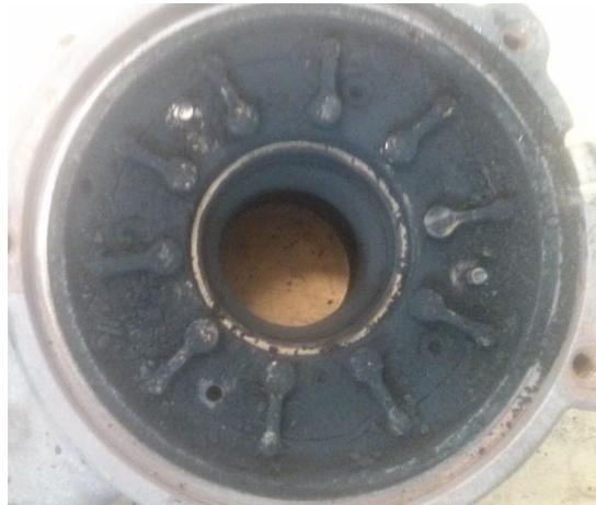
7. Remove the three TorX screws and lift the VNT assembly out of the turbo.
