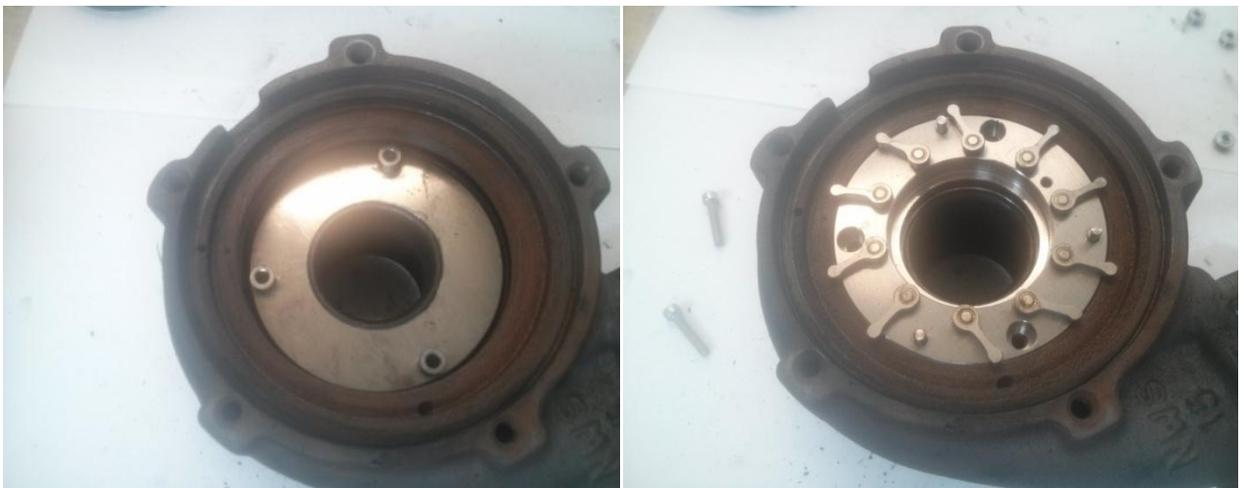
11. Carefully lower the vanes down on to the spacers making sure they don't move. It will only fit in one orientation as the holes are off centred. Drop the screws in and tighten.
