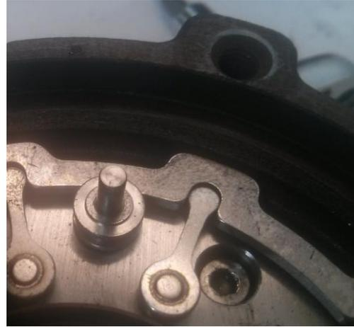
13. Once the control ring is seated flat, lift it just a little and then push the rollers in to place. Push the pins in to fix them in.
