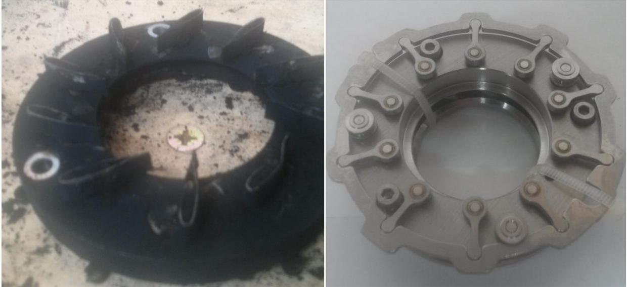
8. Inspect the vanes for damage. If any are bent or melted they need to be replaced. If they are damaged, carefully inspect the turbine wheel to ensure there have been no collisions.
